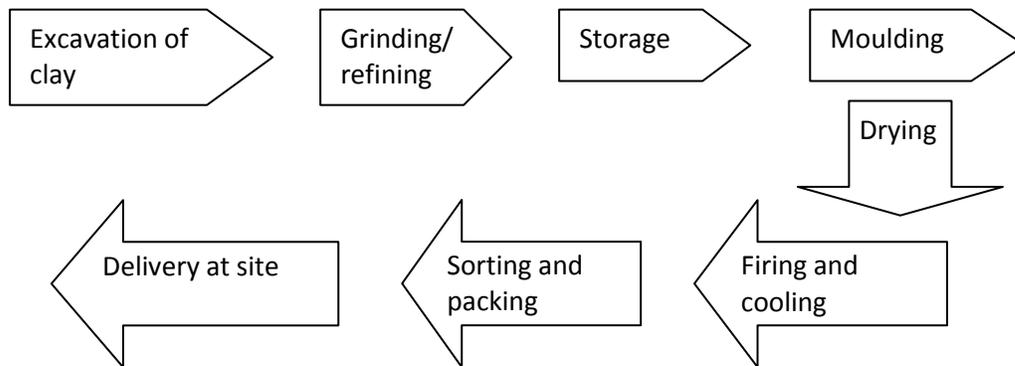
Figure 2 Lobatse Clay Works manufacturing process
