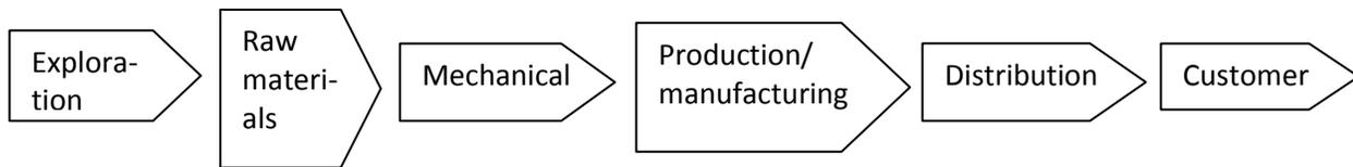
Figure 1 Process flow for clay brick manufacturing
