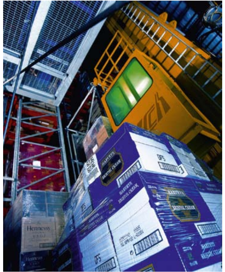
A pallet of goods being transferred by crane to conveyor belt in the YCH ASRS facility.
