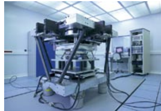
The self-designed LNE Nanometer Reference Measuring Machine combines a 300\text{mm} \times 300\text{mm} \times 50 \mu\text{m} measuring volume with the AFM technology in a clean room facility and a very stable and controlled environment. All X, Y, Z displacement is traceable to SI units by laser interferometry.
