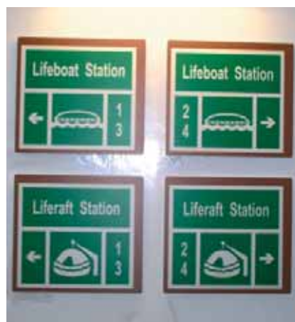
Good directional signs can help reduce the time needed to evacuate a ship.
