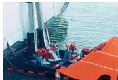
Marine evacuation systems chutes are used to evacuate a large number of people within a 30-minute evacuation time.
