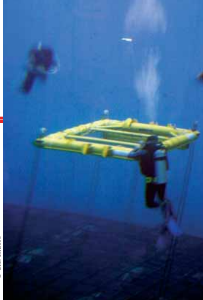
Testing a riser-sustaining buoy in the test tank in the oceanic technology laboratory.
