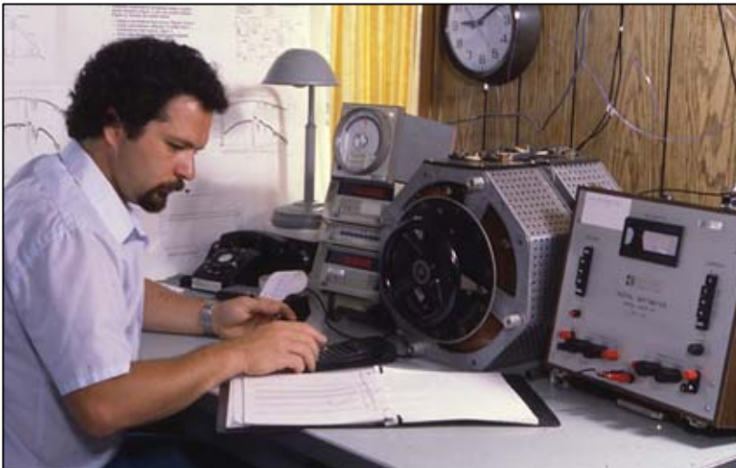
Power Input to Electric Strip Heaters Manually Adjusted to Replicate Absorbed Solar irradiance – NBS 1981
