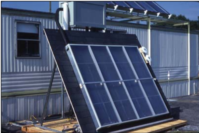
Refrigerant Charged Solar Hot Water System Evaluated Outdoors at NBS and Indoors at National Solar Test Facility in Canada
